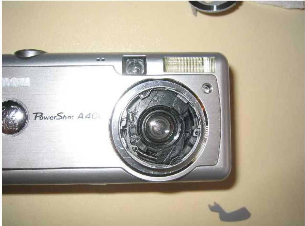
Carefully reinsert the lens cover springs using tweezers or in my case a magnetized screwdriver. Then reinsert the lens covers, inserting their pins into their support holes in the lens cover mechanism and the lens cover springs. Note that with the lens barrel open, the lens covers should now easily install in the open position.
