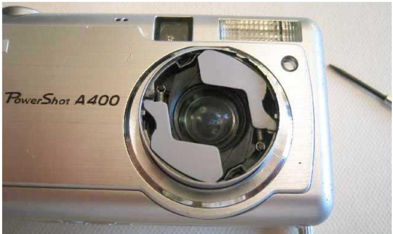
Now apply very small dabs of glue (I used super glue) to the glue tabs on the silver ring. A little bit of glue should easily suffice. Remember that you may need to get in there again someday. Now simply reinsert the silver ring onto the barrel. Your camera is now repaired. Reinsert the batteries and verify proper operation. This particular camera is now going to my niece as her first digital camera!
