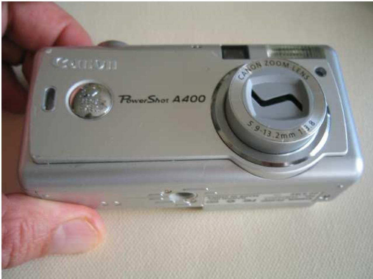
With the camera powered on and the lens extended, remove the camera's batteries. The lens should remain extended.
