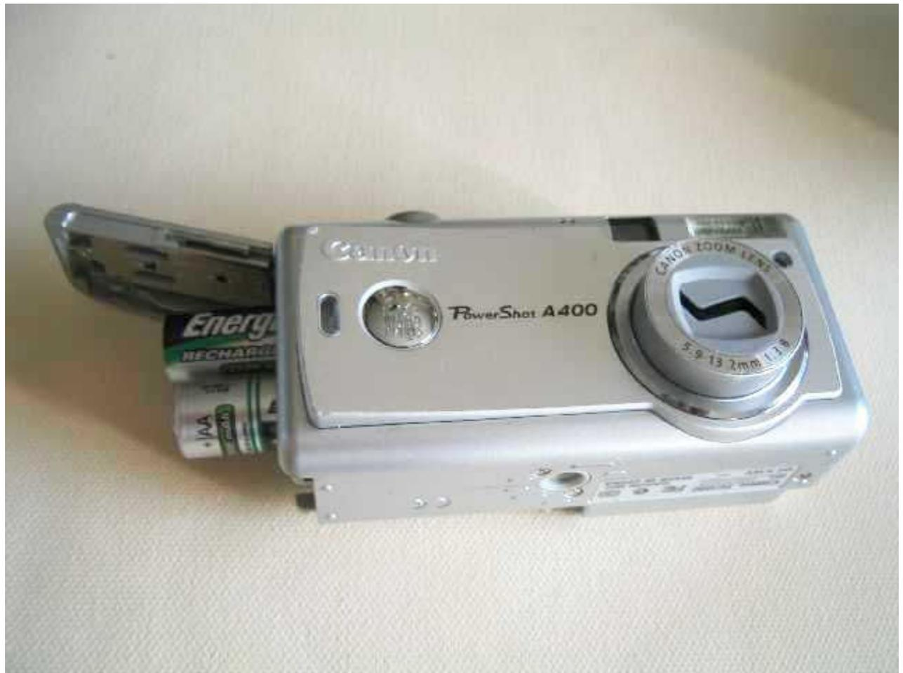
The lens cover mechanism is accessible by removing the silver band ring on the front of the lens mechanism. This is true for most Canon digital cameras (suspect this is also the same for other brands). The trick is how to remove that silver band. To do so you'll need a Q-tip, some rubbing alcohol, and the pointy tip from a box cutter.
