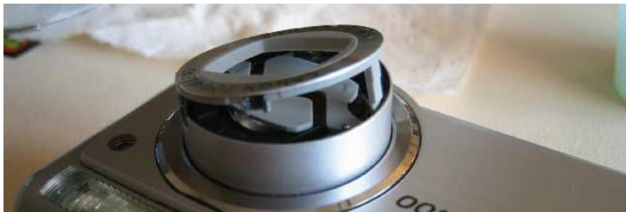
Now closely inspect the exposed lens cover mechanism to note how it is assembled. If you have another camera, recommend taking a couple macro pictures to help you remember. In the below picture, note that the black lens cover opening mechanism is not fully resting against its metal stops (at the eleven and five o'clock positions) even though the lens barrel is fully extended.
